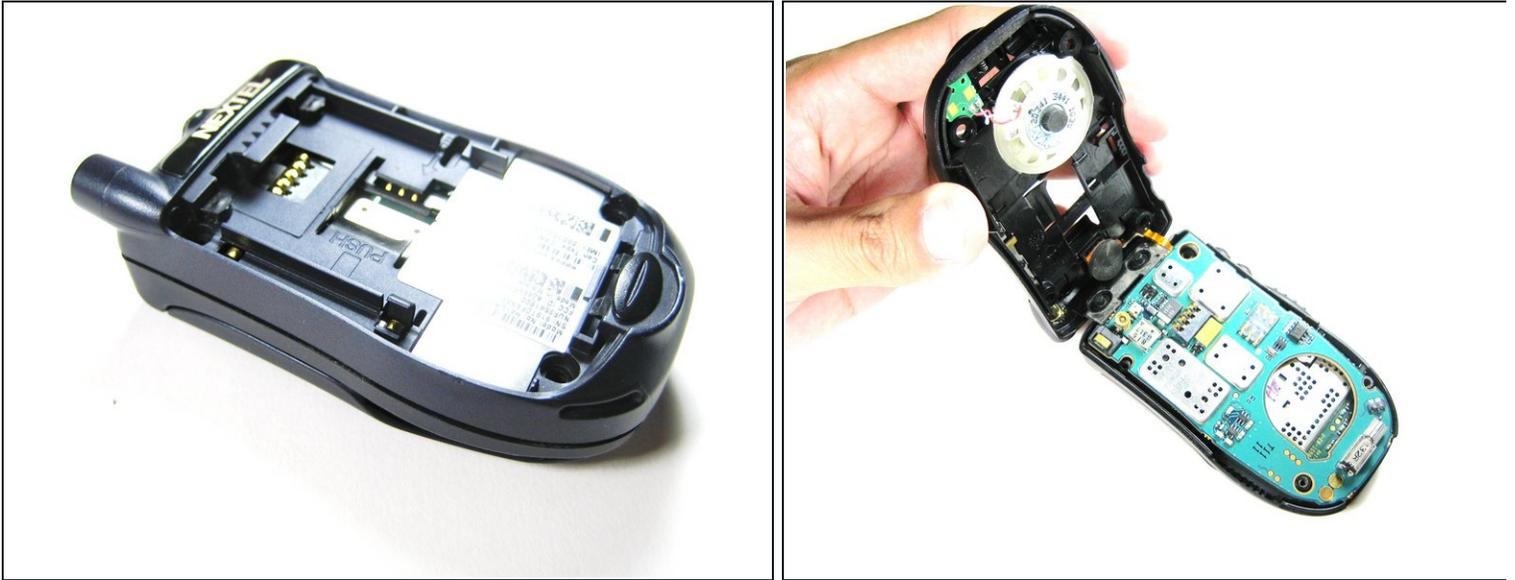
**⚠ DO NOT force the cover off as it could damage the ribbon cable!**
