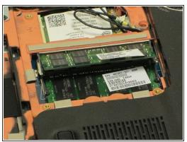
Locate the grey clips on the side of the RAM and pull the grey clips away from the RAM using the plastic opening tool.
