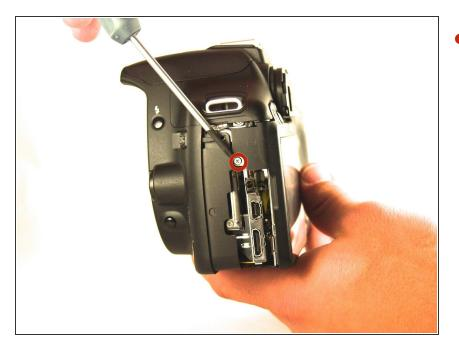
Unscrew the inner 4mm screw with a #00 Phillips screwdriver.
