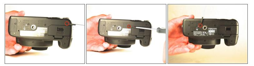
Unscrew the bottom three 4mm screws with a #00 Phillips screwdriver.
