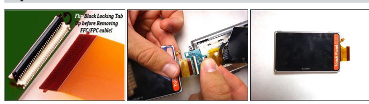
• Use a spudger or plastic opening tool to flip the black locking tab up. Slide the cable straight out of its socket and remove the display.
