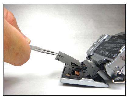
Remove black plate with tweezers. (Be careful not to lose the small square magnet sticking to the underside. It allows the auto rotation of the screen for selfies.)
