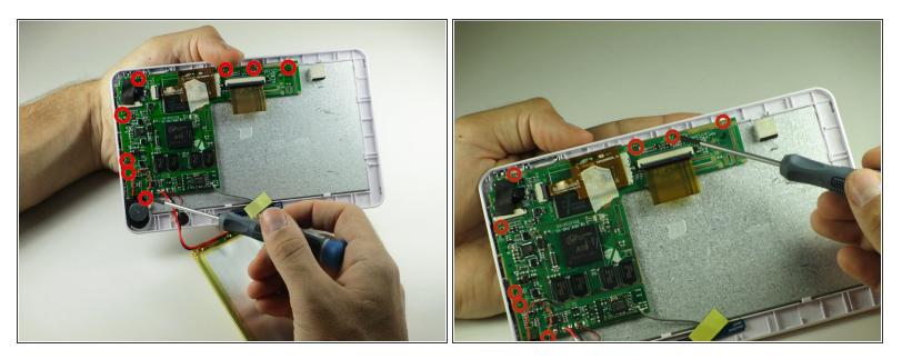
Use a Phillips #00 screwdriver to remove the eight 40mm screws holding the motherboard in place.
