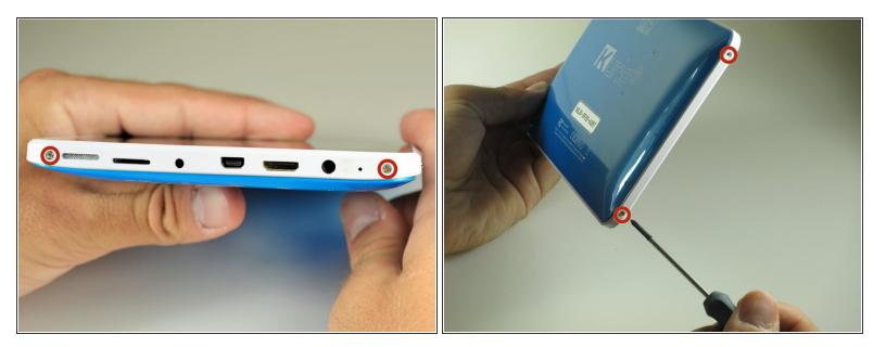
• Remove the four 30 mm Phillips #00 screws from the outer case.
