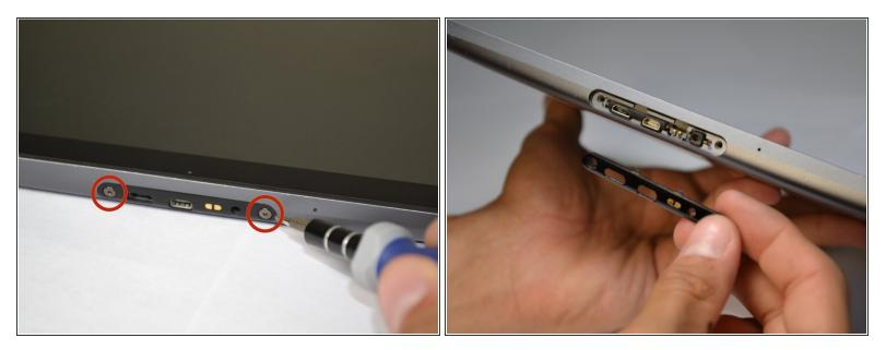
There are two 6.6 mm screws that hold ports into place as well as the back panel. Remove these with a T5 Torx screwdriver.
