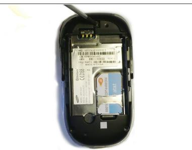
Remove the five screws with a size 00 screwdriver. There 4 in the corners and one on the top as shown.
