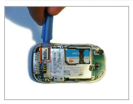
Detach the tab from the logic board by using iPod Opening Tool (as shown).
