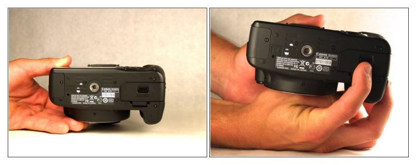
• On the bottom of the device, use your fingers to push down on the latch on the battery door.
