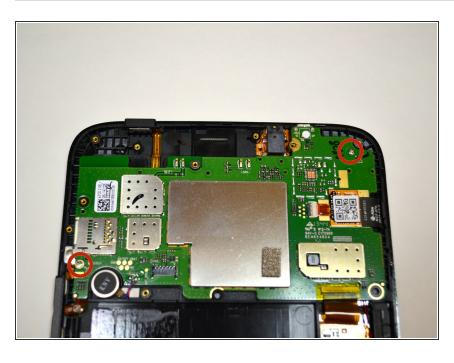
Using a #000 Phillips screwdriver, remove the two M1.4 3.5mm screws from the system board and set them aside.
