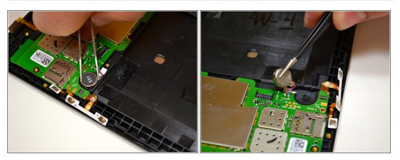
• Remove the circular motor unit by gently pulling up on it using a tweezer.
