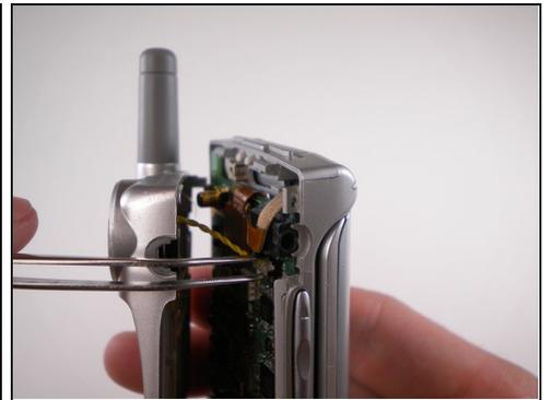
⚠ When removing back cover, be careful not to break the speaker wires.
