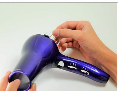
Using your index finger push the fan grill down with moderate force.
