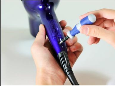
Remove the two 15.875 mm Phillips #2 screws from the back panel.
