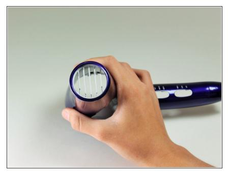
Hold the front panel of the hair dryer by the nozzle facing upward.
