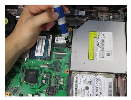
Use a Phillips #0 screwdriver to unscrew one 0.6 mm screw located just to the left of the disc drive.
