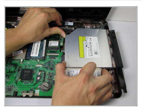
Position your thumbs to push firmly and slide the disc drive to the right through the rectangular hole in the side of the laptop and out.
