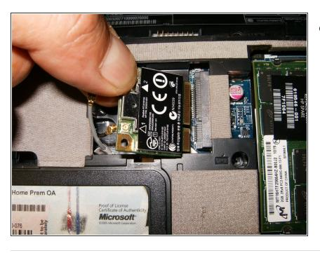
Remove the WLAN module by pulling it away from the slot at an angle.
