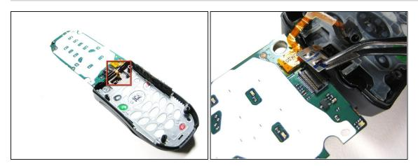
• Using tweezers, carefully pull off the connector shown.
