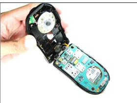
⚠ DO NOT force the cover off as it could damage the ribbon cable!
