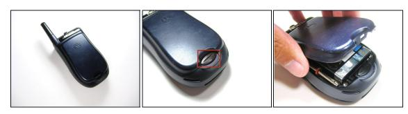
• Slide the notch downward while pulling the back cover off to remove it.
