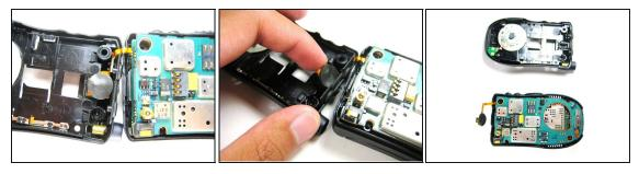
• Carefully pry off the connection between the headphone jack and logic board.
