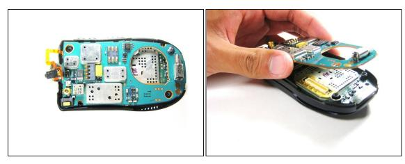
• Lift the first logic board off of the rest of the device.
