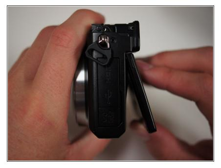
• Lift the LCD screen with your fingers such that the screen is bent slightly away from the camera.
