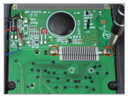
Next, use a Phillips #00 screwdriver to remove the two screws located on each side of the striped ribbon between the two green circuit boards.
