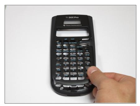
Pry the front cover off of the calculator with a prying tool from the bottom up.
