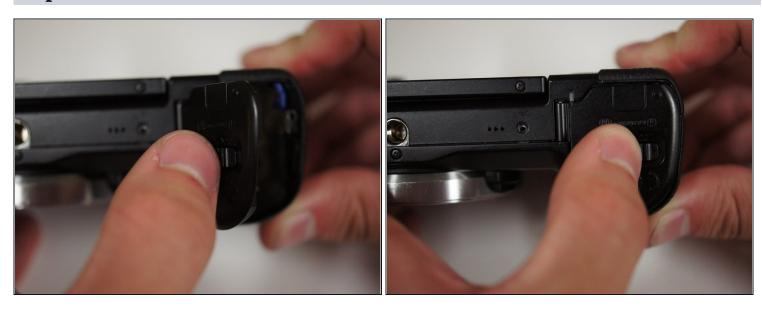
• Close the battery door by pushing it down until it latches shut.
