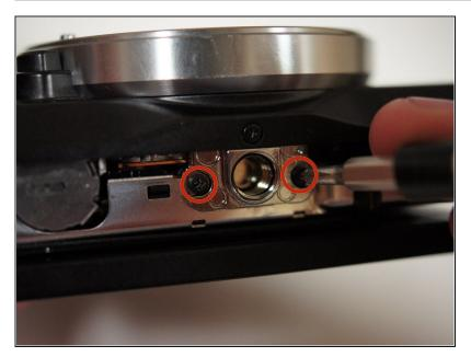
Remove two more 3/32" #00 screws from the bottom of the camera using the Phillips #00 screwdriver.
