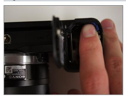
With the battery door open, push the blue lever in the battery compartment to release the battery.
