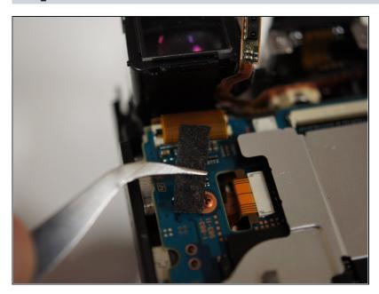
Using the tweezers lift the black piece of tape from the circuit board below the viewfinder.
