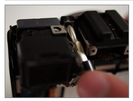
Remove the 5/32" #00 screw next to the back right of the viewfinder using the Phillips #00 screwdriver.
