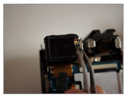
Using the <u>tweezers</u>, unhook the flexible circuit board from the metal tab on the right of the viewfinder by rotating it to the left.
