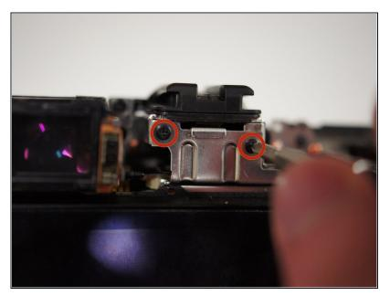
Remove the two 3/32" #00 screws located next to the viewfinder using the Phillips #00 screwdriver.
