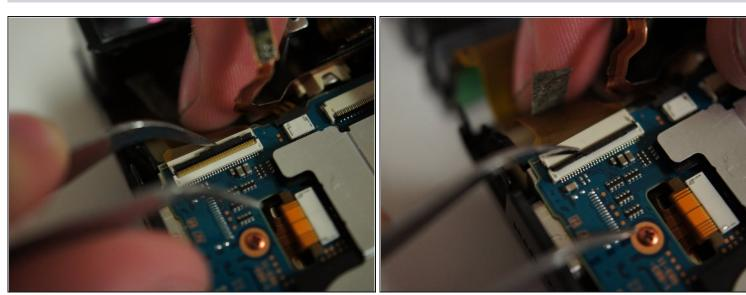
• Use the tweezers to lift the black switch on the white receptacle just below the viewfinder. If properly opened, the ribbon cable will remove with very little force.
