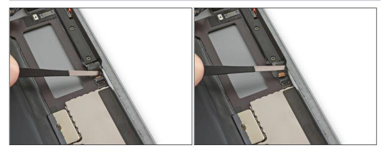
• Slide the upper button assembly cable straight out of its ZIF connector.
