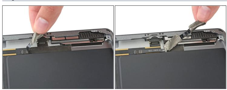
• Remove the tape covering the left speaker cable connector.
