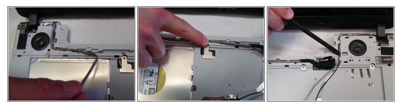
• Place the power and display cables for the new screen into their respective grooves.
