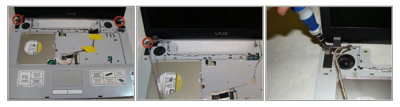
• Use a Phillips #0 screwdriver to remove the two screws (Length: 6.9 mm) that attach the screen to the body of the laptop.
