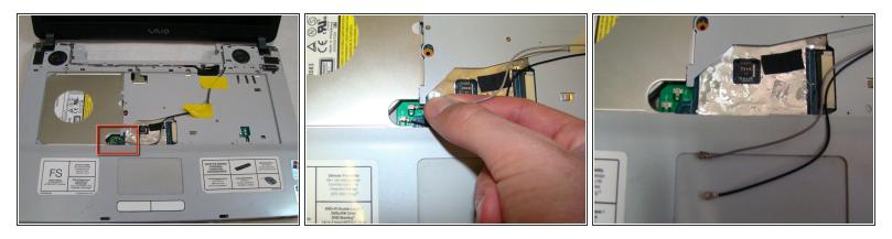
Use your fingers to pull the LCD screen's display cables away from their connections.
