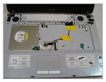
At this point the speaker cover and keyboard should be removed and the laptop should be sitting in its normal open position with the screen facing you.
