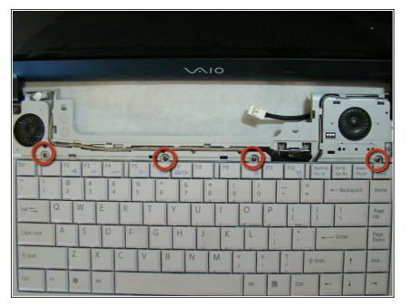
After removing the speaker cover, remove the four screws (Length: 3.6 mm) with your Phillips #0 screwdriver that hold the keyboard in place.
