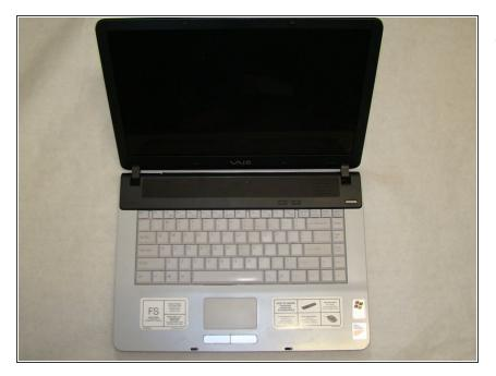
After the screws are removed, flip the laptop over so the keyboard is facing up and move the screen to its upright position.
