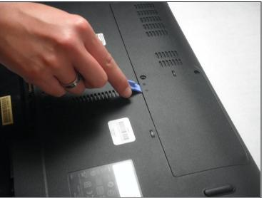
Once both screws have been removed use a plastic opening tool to lift the panel up. Starting
