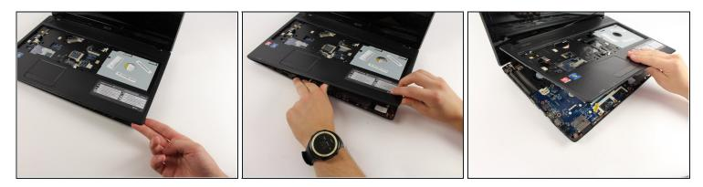
• Carefully lift up the corner of the top panel of the laptop. Once it starts coming off continue to lift it while holding the open side with the other hand.
