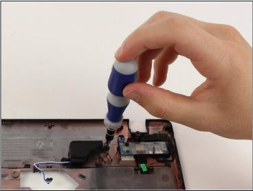
Locate and remove the two screws to loosen the speaker from the panel.
