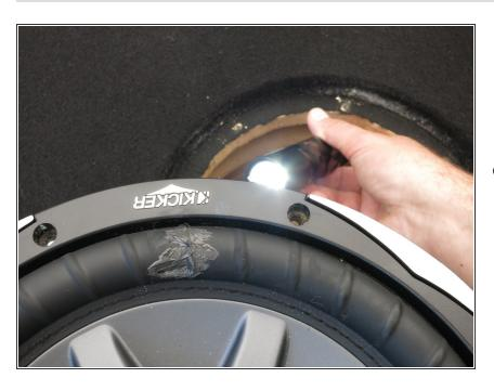
After you're done applying the RTV silicone and testing the subwoofer's excursion, shine a strong flashlight
