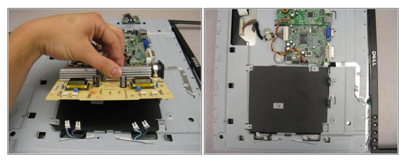
• The power supply board can now be removed.
