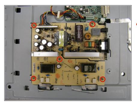
Remove the five 7 mm Phillips #2 screws from the power supply board.
