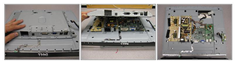
• Lift up on the back panel to remove it from the rest of the monitor.
