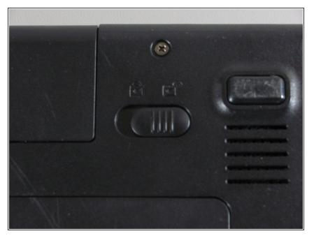
Move the latch to the right of the battery to unlock.
