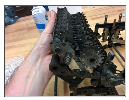
Remove the driver wheel assembly.
