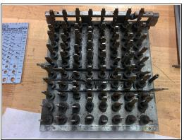
• The lockbars have springs attached to them. Remove the lockbars by unhooking the spring end on the lockbar side first. Leave the springs attached to the base plate for now.
