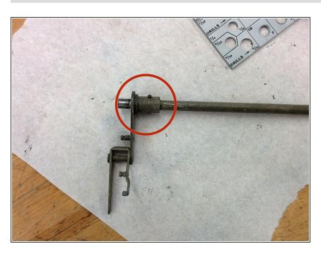
Remove taper pin and part from the other end of the shaft.
