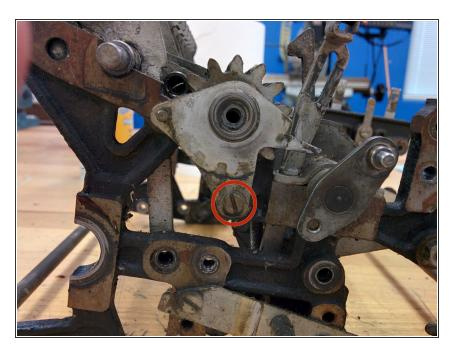
Remove this screw, #8-36, 1/2", along with its plate and the washer, 5/16" od, 1/8" thick, that is between the plate and the frame.
