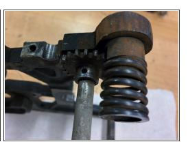
Now, assuming that the arbor press did move the pin, you can gently knock the pin out with a 1/16" flat pin punch and a hammer.
