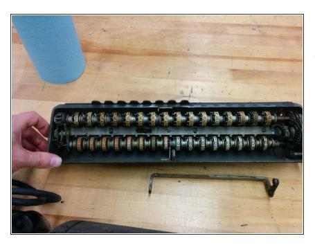
The underside of the carriage, and the other part. The shaft is not shown. Put all of these into a box so they don't disappear.
