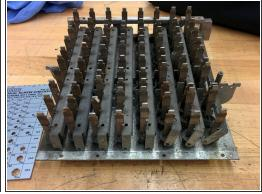
Turn the keyboard assembly over, and remove the frame by lifting up a bit and then out. There are pins on the frame which allow lock bars for each row to pivot.
