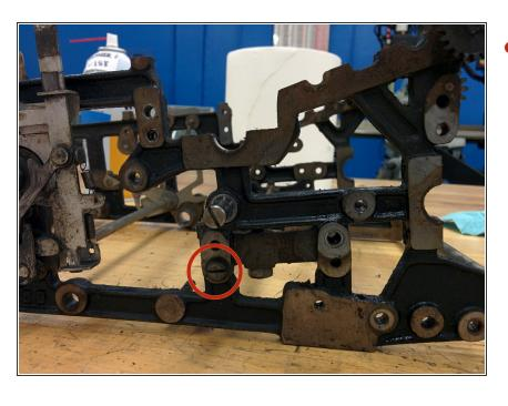
On the left side, remove this screw, 3/16-32 x 5/8" and split washer, 5/16" od x 0.085".
