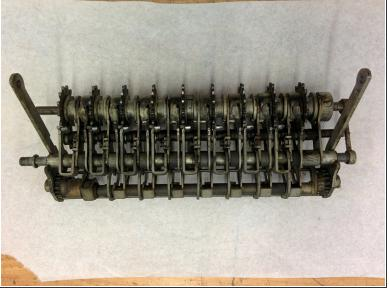
Now we'll disassemble the intermediate gear assembly.
