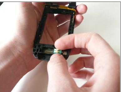
Remove the black sim card reader and green vibrator before continuing to ensure they do not fall out.
