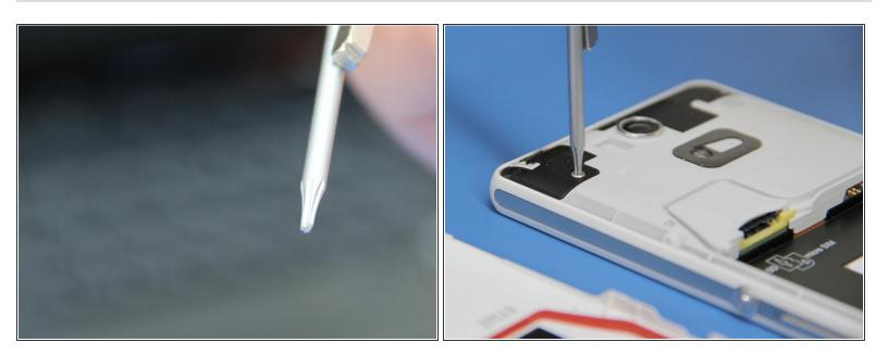
Use T6 Torx Screwdriver to remove all screws you can see on the back panel.
