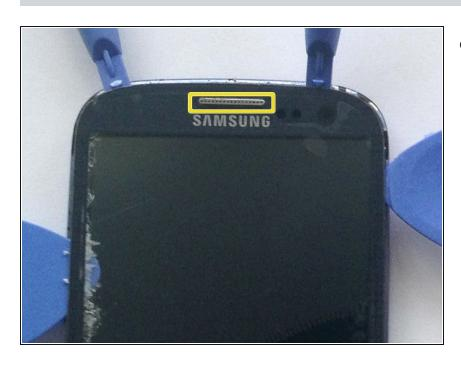
Remove this little piece of metal from your old glass, it will need to be inserted into the new one.
