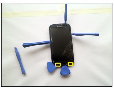
↑ You should start to separate the glass from the top edge, gradually moving towards the center, peeling off the entire screen from top to
