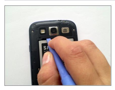
Take out the battery. It has no adhesive or wires attached to it.
