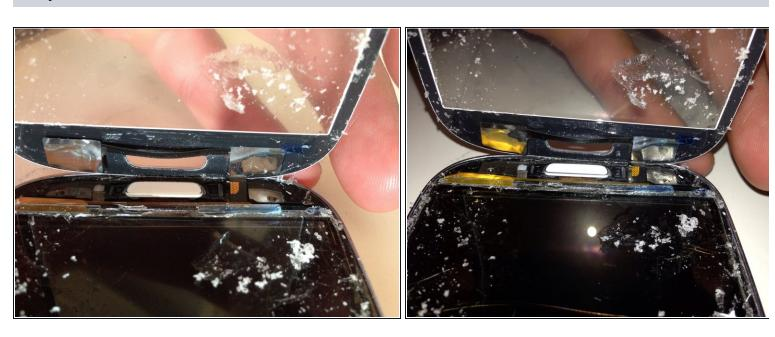
At this step, you need to be very careful not to damage the buttons or cable! Using a spudger, separate the buttons from the inside of the glass. It may need to be warmed up a bit. Perhaps the best option is to start in the middle, under the middle cable connecting the two buttons, then separate each button.
