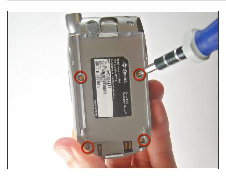
Unscrew the four screws behind the battery
