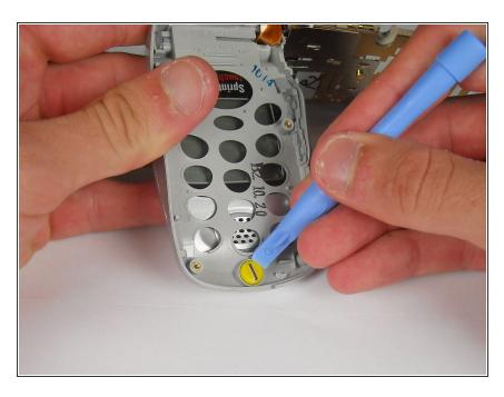
Pry out microphone with opening tool
