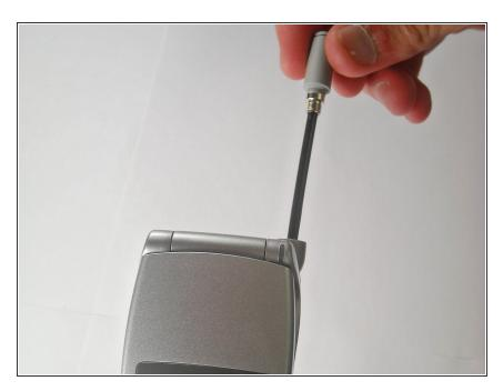
Unscrew and remove antenna from socket
