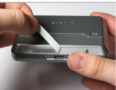
Peel off the sticker from the bottom of the device to reveal two screws.
