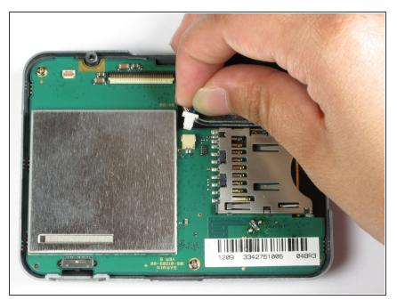
Pull out the cable between the logic board and the speaker to disconnect them.
