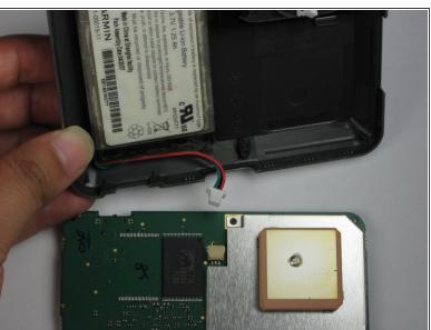
Detach the logic board form the battery by pulling out the cable.
