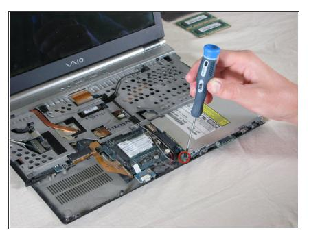
• Remove the securing screw on the bottom left of the optical drive.
