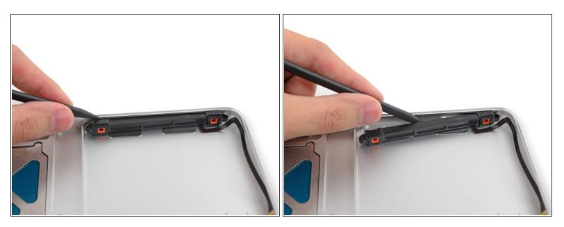
Insert the tip of the spudger between the hard drive bracket and the front edge of the upper case to free it from its recess.
