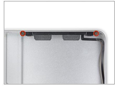
Remove the two 5 mm Phillips #00 screws securing the hard drive bracket to the upper case.
