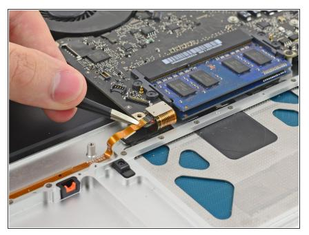
• Pull the hard drive bracket cable out of its socket.
