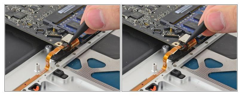
• Use the pointed end of a spudger to flip the lock on the ZIF connector.
