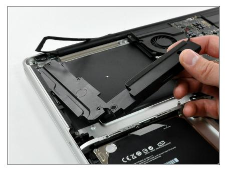
• Lift the subwoofer and right speaker assembly out of the upper case.
