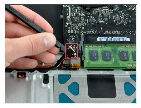
• Use a spudger to pry the hard drive cable connector straight up off the logic board.
