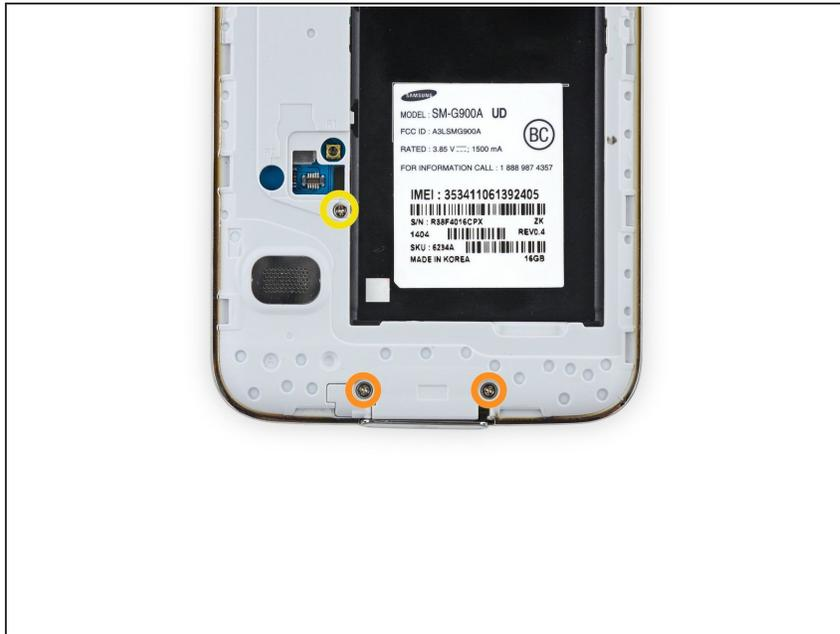
**i** Flip the phone over and remove the following screws from the battery side of the midframe:
