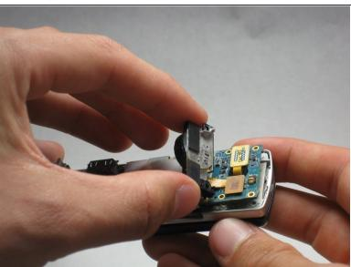
Use the iFixit opening tool to remove the camera/speaker from the motherboard.
