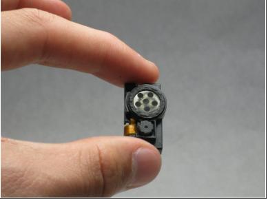
• Use the iFixit opening tool to gently pry the camera/speaker off.
