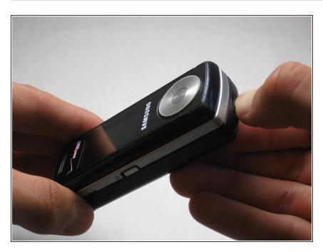
Press and hold down the button on the bottom side of the phone with your finger.
