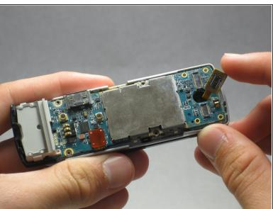
Use the iFixit opening tool to remove the yellow tab on the motherboard.
