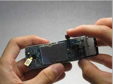
• Use the iFixit opening tool to remove the other orange tab to free the motherboard.
