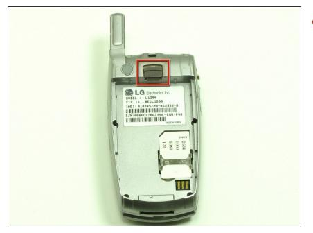
Remove the battery from the back of the phone by lifting up the tab.
