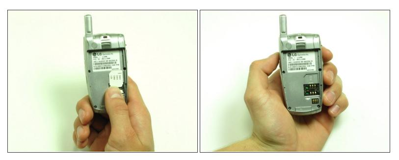
• Push the SIM Card up using your thumb until it is removed.
