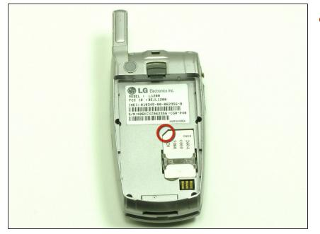
Once removed, replace with new SIM Card, making sure that the cut corner fits into the cut corner of the slot.
