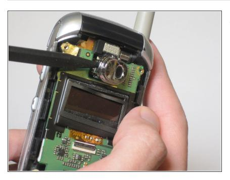
• Use a spudger to remove the plastic camera casing.
