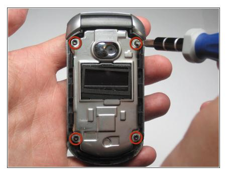
• Use a T6 Torx Screwdriver to remove all 4 small screws.
