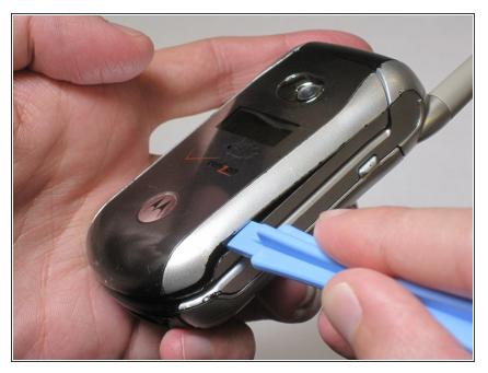
Place a plastic opening tool in the small crack that runs along the side of the front case to pry it off.
