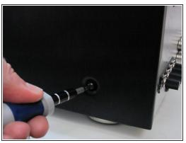
Remove the two screws on both sides of the receiver. Keep these and the rest of the screws in a safe place.
