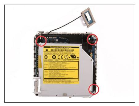
Remove the three black Phillips screws securing the plastic framework to the logic board and lower case.
