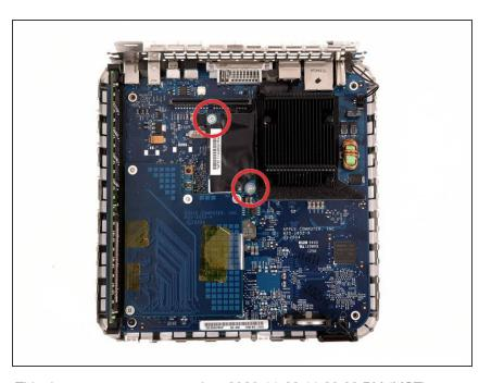
Remove the two silver Phillips screws from the corners of the modem board.
