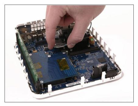
Pull the modem up from its connector. If it sticks, just wiggle it back and forth a bit as you pull up.
