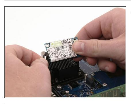
Disconnect the RJ-11 cable from the back of the modem.
