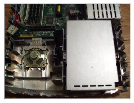
To remove the floppy, pull on one clip, and lift the drive. Then release the other and the drive should come free. Remember to disconnect the data cable.
