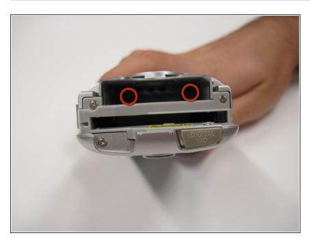
Remove two 4.5 mm screws from inside the battery slot.
