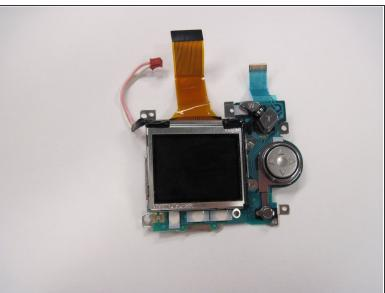
Gently lift the LED screen out of the remaining casing and set it aside.
