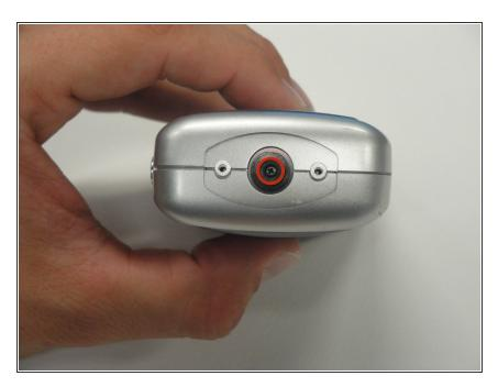
Remove the plastic cap and the 5 mm screw underneath.
