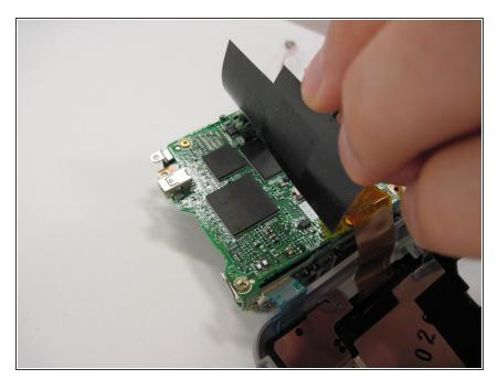
Lift up on the black covering and remove the orange wire connecting the lens to the motherboard.
