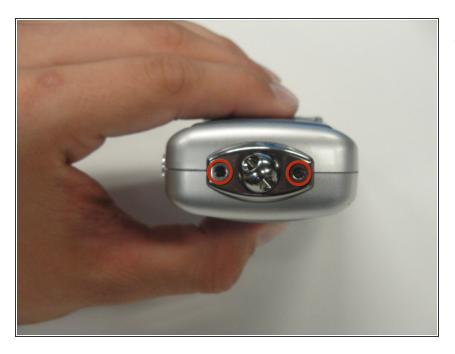
Remove two 5 mm screws from the opposite end of the battery slot.
