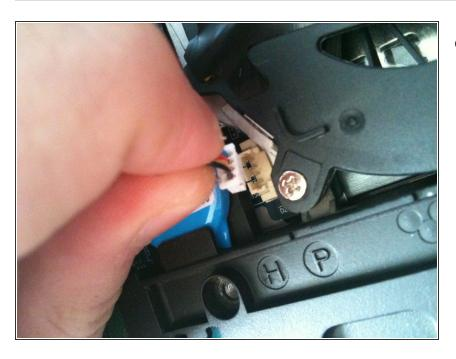
Pull the fan cable straight away from its socket.
