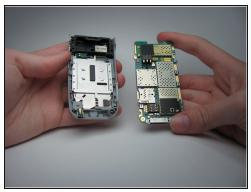
Remove the logic board from the bottom casing.
