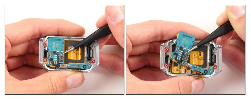
• Once the safety belt is removed, use tweezers to take the motherboard out of the Gear 2.
