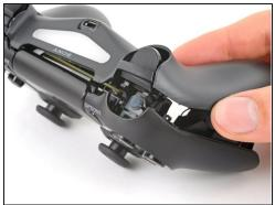
Press the R2 button and slide the rear case over it.
