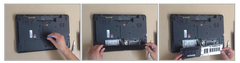
• With a plastic tool remove the Memory RAM / Hard Drive / Wifi Cover Door
