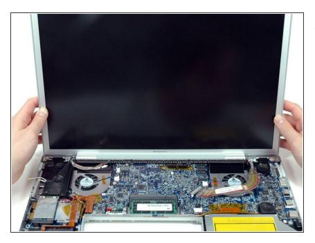
Grasp the display assembly on both sides and lift it up and out of the computer.
