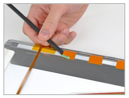
Use the flat end of a spudger to carefully peel off the three antenna straps stuck to the lower edge of the LCD.
