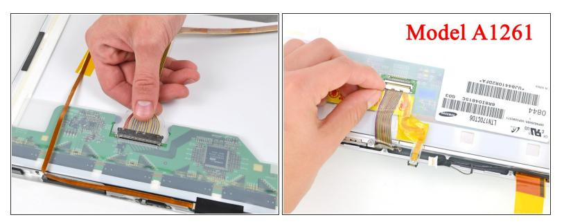
• Disconnect the display data cable from the LCD by pulling it toward the bottom edge of the display.
