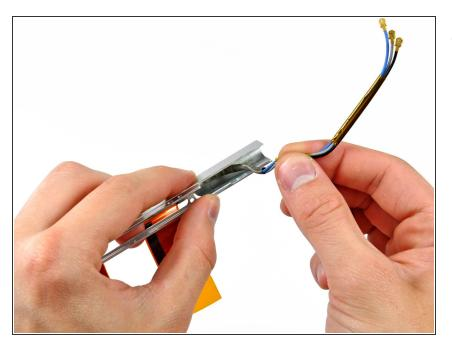
If necessary, peel the antenna leads off the adhesive securing them to the clutch cover.
