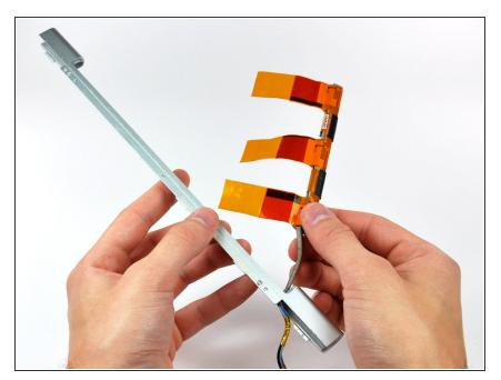
Remove the antenna cables from the clutch cover, being careful not to damage the three antenna straps.
