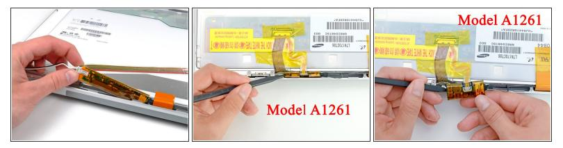
• Carefully lift the inverter out of the clutch cover.
