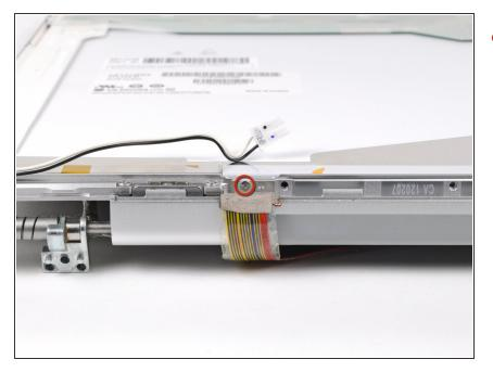
Move the display data cable out of the way to remove the Phillips screw hidden underneath.
