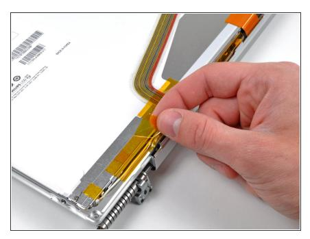
Remove the piece of tape securing the backlight cables to the front display bezel.
