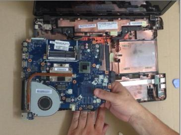
• Disconnect the Power /Charging cable connector from the back side of the Motherboard.
