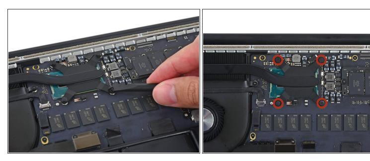
Use the flat end of a spudger to peel the four foam stickers off of the heat sink screws.
