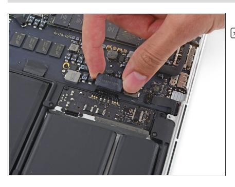
Bend the battery connector up out of the way to prevent accidental contact with its socket during your repair.
