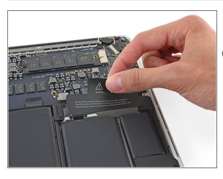
i If necessary, remove the plastic cover adhered to the battery contact board.
