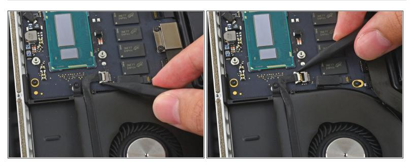
• Use the tip of a spudger to push on either side of the the iSight camera cable connector to walk it out of its socket on the logic board.
