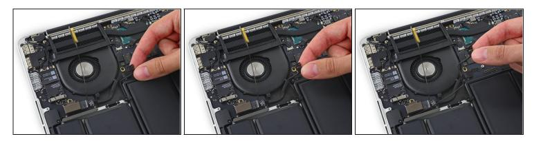
• Carefully peel the right speaker cable off the upper case.
