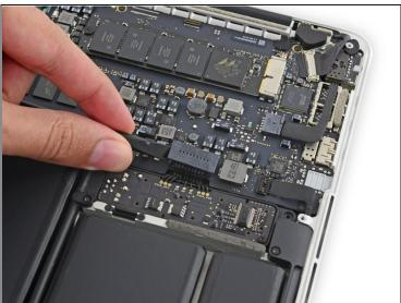
• Use the flat end of a spudger to lift the battery connector straight up out of its socket on the logic board.
