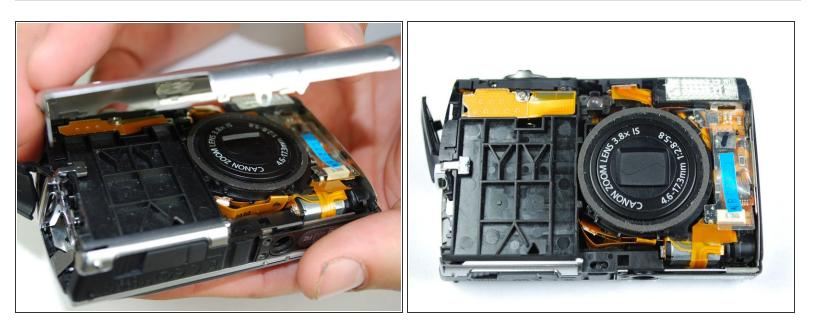
• Pull the front cover from the camera by using gentle upward pressure.
