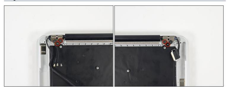
• Remove the four inner 5.3 mm T8 Torx screws (two on each side) securing the display to the upper case.
