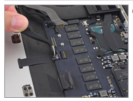
i If necessary, peel back any tape covering the trackpad cable connector.
