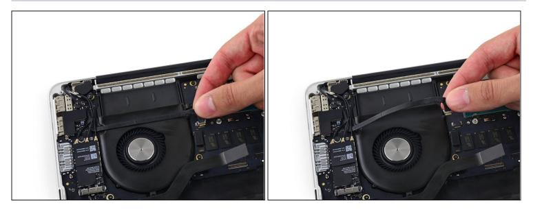
• Peel the iSight camera cable up off the fan housing to fold it out of the way.
