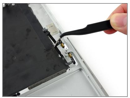
• Remove the microphone cable from the upper case.
