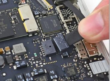
• Pull the DC-In board connector straight out of its socket on the logic board.
