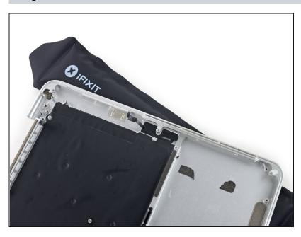
Place the MacBook on a heated iOpener for about a minute to soften the adhesive securing the dual microphone cable.
