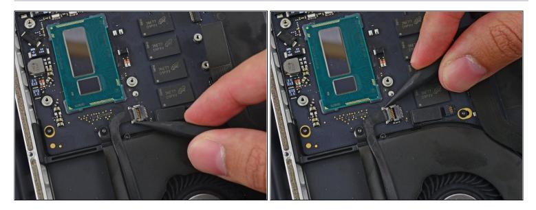
• Use the tip of a spudger to push on either side of the the iSight camera cable connector and *walk* it out of its socket on the logic board.
