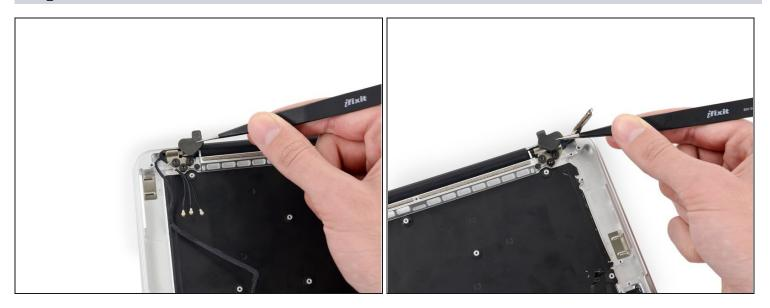
• Use a pair of <u>tweezers</u> to lift the rubber hinge covers up off the right and left display hinges.
