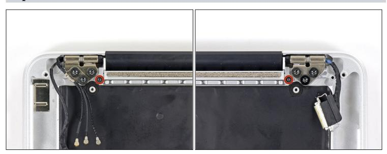
• Remove the 3.2 mm T5 Torx screws (one on each side) securing the aluminum hinge brackets to the upper case.
